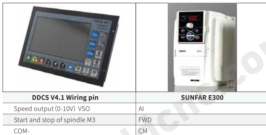
Figure 2-9 DDCS and VFD wiring
