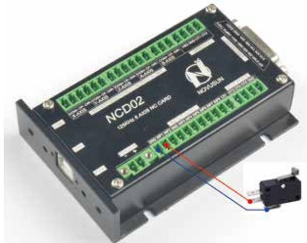
Picture 2-5 2 Lines Proximity Switch Connection Method
