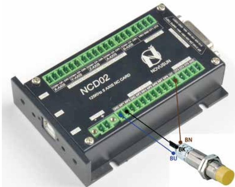
Picture 2-7 NPN 3 lines Proximity Switch example
