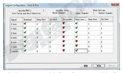
This page is to select the stepper motor control pins. Because Stepper motor control pins address are fixed by the controller board, So here only need to define the Pin address(No.s), we can define other parameters meter. To make sure the Z axis to the right direction(Up is '+',down is '-'), Z axis's "Dir low" should be set to " $\sqrt{}$ ". Other axes's should be set as the user's request.
