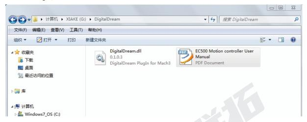
In your computer which you will run the EC300 controller, you must already installed the Mach 3 Software, and now pls copy the PlugIn in to C:\Mach3\PlugIn.(If the user install the Mach 3 software in C-disk.)
