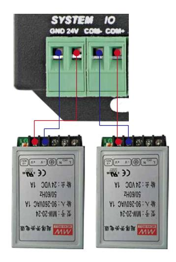
Figure 5-13 Power supply for Controler System and for IO Port
