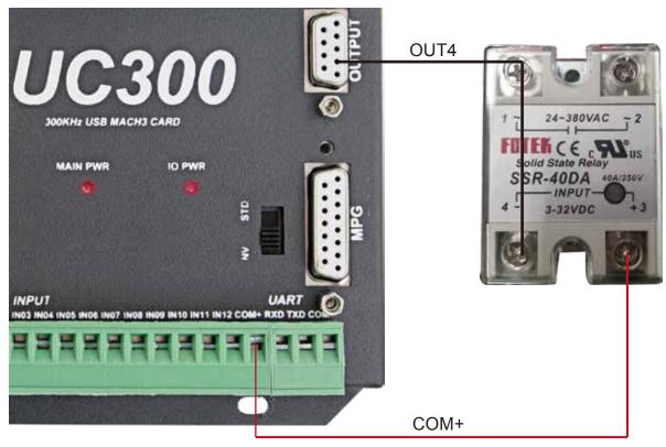
Figure 5-7 Solid Replay Connection
