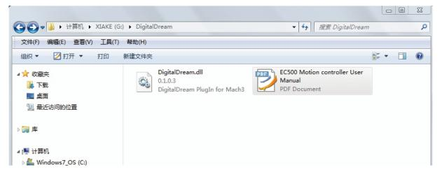
In your computer which you will run the UC300 controller, you must already installed the Mach 3 Software, and now pls copy the PlugIn in to C:\Mach3\PlugIn.(If the user install the Mach 3 software in C-disk.)
