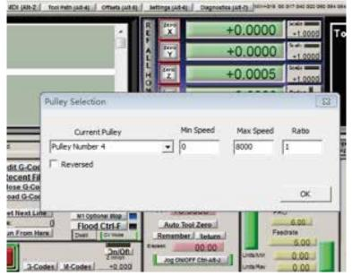
Figure 5-4 UC300 Spindle Motor Max Speed Setting
