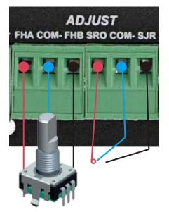
From the Figure 5-1 shows, the Marked No. 9 is for adjustable input interface, which must be operated by the digital potentiometer. The interface will make us to operate the FRO, SRO and SJR very Easy and convenient. The Interface should be operated with position switch and digital potentiometer, for the FRO, SRO and SJR adjustment.
