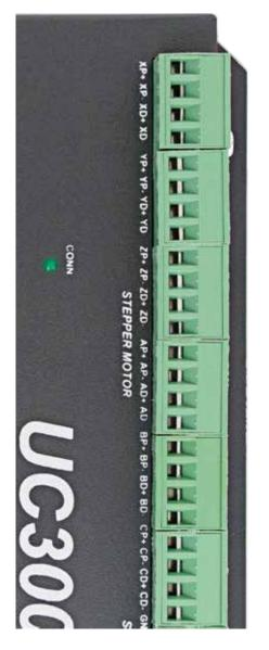
As the Marked No. 2 from Figure 5-2, there is the Stepper/Servo Interface. The device can be used to control machine tools with stepper or servo motor controls with pulse and direction signals. The option for users is 3-6 axis.
