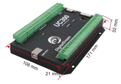
Figure 3-1 UC300 Front Appearance and size
