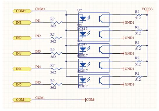
Figure 5-9 Internal structure of Input interface
