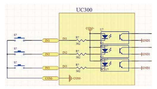
Figure 5-10 Probe/Estop/ and other switch input connection
