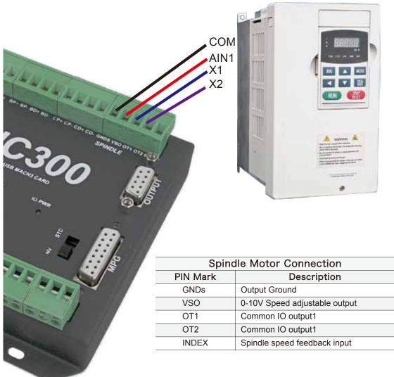
Figure 5-3 UC300 Spindle Control Setup
