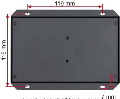
Figure 3-2 UC300 Installation Dimensions
