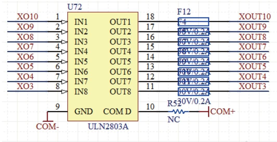
Figure 5-9 OUTPUT port internal structure
