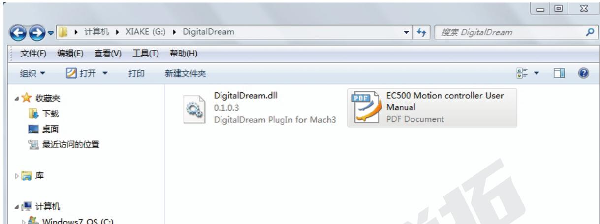
In your computer which you will run the EC300 controller, you must already installed the Mach 3 Software, and now pls copy the PlugIn in to C:\Mach3\PlugIn. (If the user install the Mach 3 software in C-disk.)
