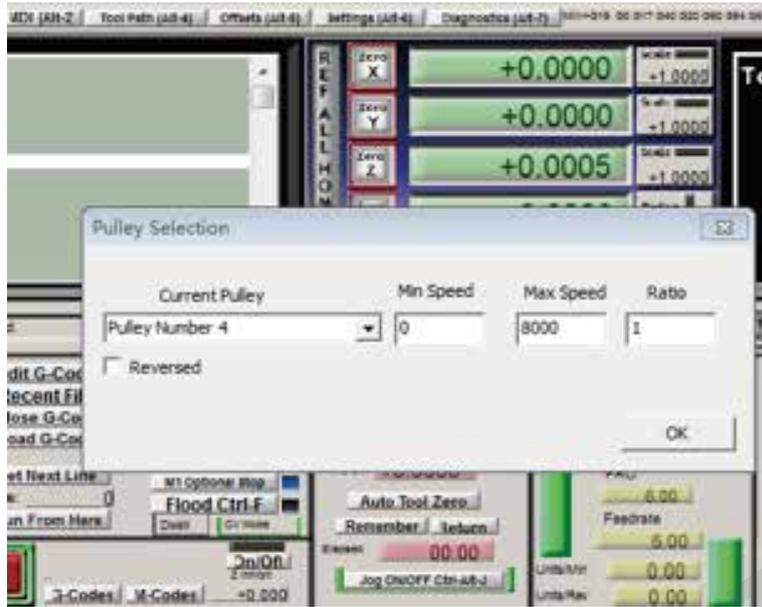
Figure 5-7 EC300 Spindle Motor Max Speed Setting
