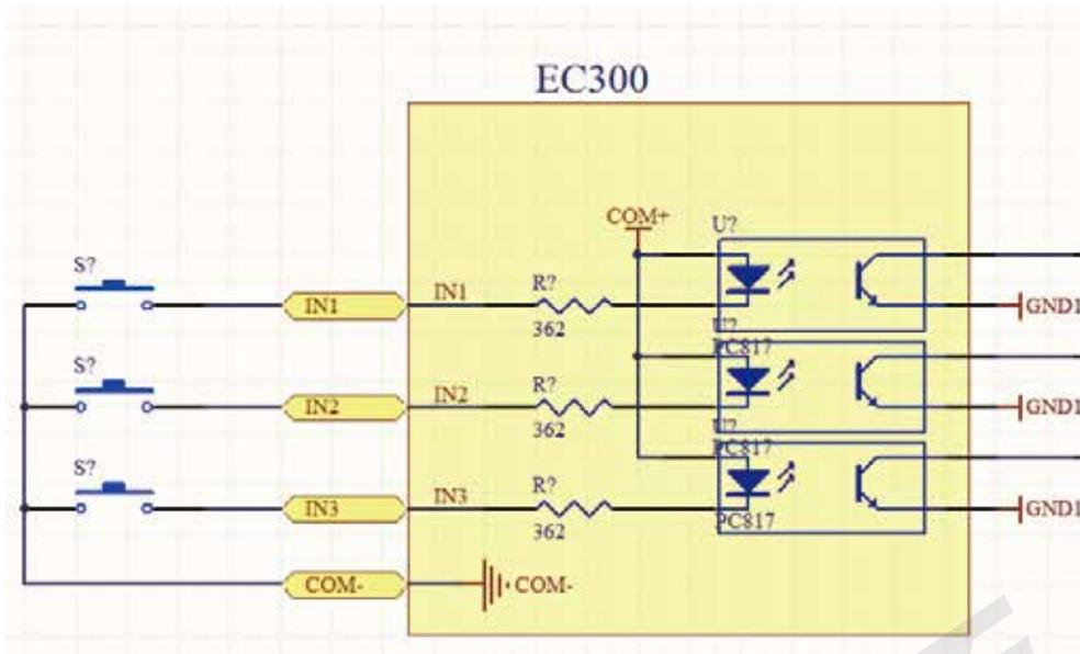
Figure 5-13 Probe/Estop/ and other switch input connection
