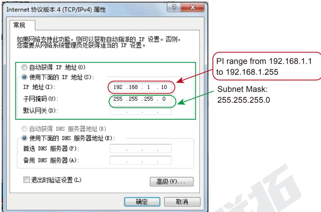
Figure 5-3 EC300 Ethernet Communication Setup IP No.
