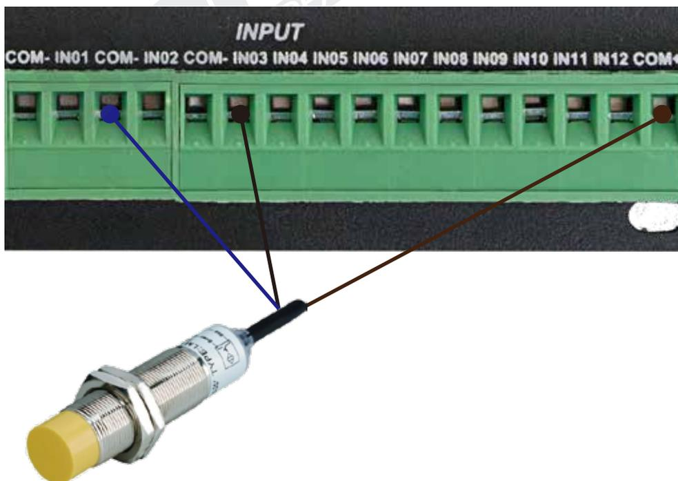
Figure 5-15 NPN 3 lines Proximity Switch Connection Example
